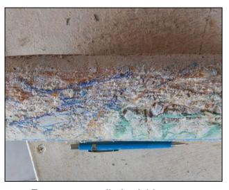
Fracture controlled soluble copper
