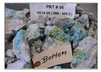
Soluble copper remaining to be recovered from pressure leach test
