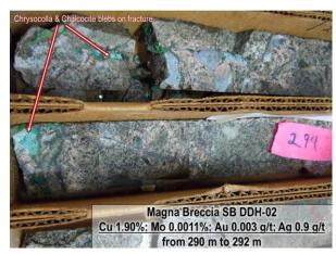
Copper mineralization in Magma breccia
