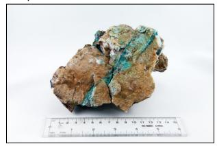
Fracture controlled copper mineralization in potassic altered Quartz Monzonite
