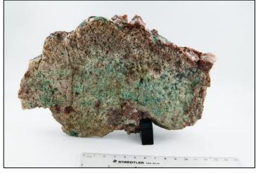
Quartz vein style copper mineralization
